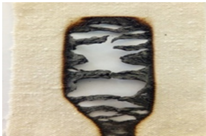
45° inclined flammability test of control Eri fabric
