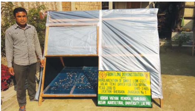
Figure 6.13. Demonstration on Low cost Solar Tent Dryer by KVK, Udalguri
