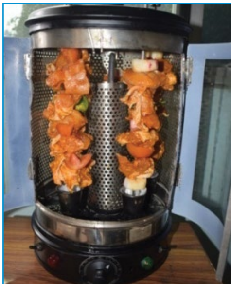
Figure 5.28. Electrically operated revolving barbecue
